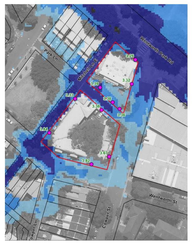
Figure 5: 1per cent AEP peak flood depth
